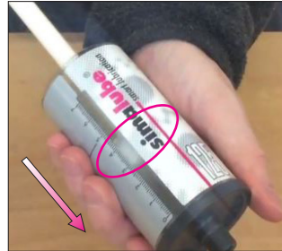
Push piston all the way down to the grey end
