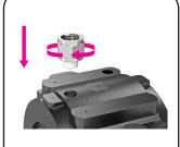
Screw in reducing nipple (Seal thread with sealing tape or other sealant)
