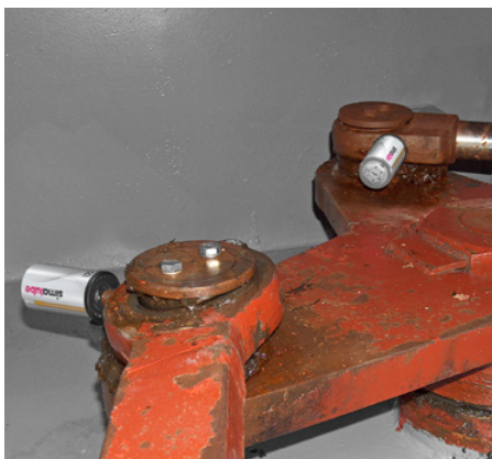
The steering wheel is lubricated with two 125 ml lubricators.
