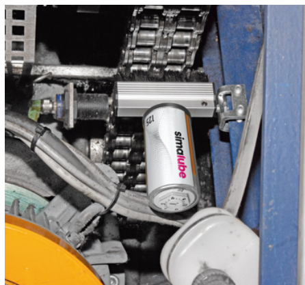
The simalube lubricator continuously oils chain, even in tight spaces. Additionally, the brush cleans the chain.
