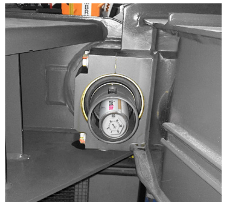
The coupling of two railway cars is lubricated with a simalube 125 ml lubricator.
