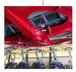
In the valley station, the deflection roller of a chairlift is lubricated with two simulube 250 ml lubricators.
