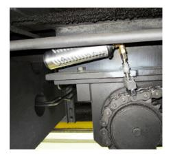
The 250 ml simalube lubricator lubricates the chain drive of a railway crane. The dispenser is also protected by a protective cover.
