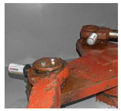
The steering wheel is lubricated with two  $125\,\mathrm{ml}$  lubricators.
