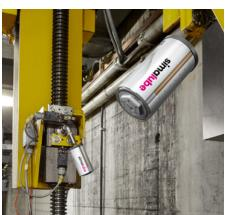
The spindles of a lifting station for railway wagons and locomotives are lubricated with 125 ml simulube over 12 months.
