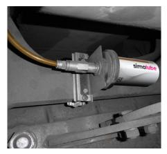
The  $125\,\mathrm{ml}$  dispenser is installed on the chassis of a low floor tram. The lubricant is directed through a hose to the lubrication point.
