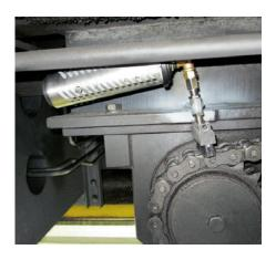
The simulube 250 ml lubricant dispenser lubricates the drive chain of a rail crane. A protective cover protects the dispenser.
