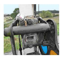
The plain bearing of a railway signal is automatically and continuously lubricated by a 30 ml simalube lubricator.
