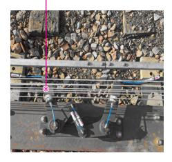
Two 30 ml simalube lubricators and four 15 ml simalube dispensers continuously lubricate the compensator of a signalling system.
