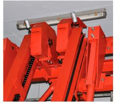
Chain lubrication with simalube on a bar screen equipped with brushes.
