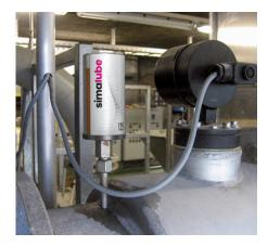
Lubricating bearings: the lubricant is transported to the bearings via a short pipe.
