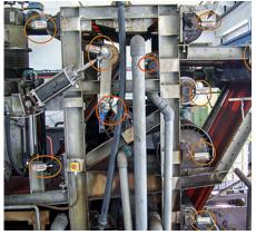
Belt filter press with dozens of lubrication points supplied with simalube lubrication.
