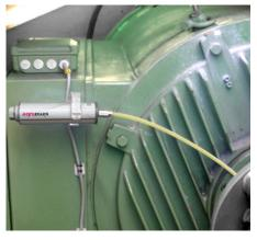
With the simalube 250 ml lubricator, the generator is continuously supplied with lubricant for up to 12 months.
