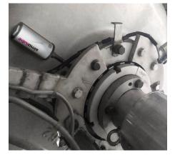
With the practical simalube accessories, it is possible to easily equip each lubrication point with a simalube dispenser.
