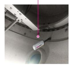
Automatic lubrication using the simalube 125 ml on a rotor blade bearing.
