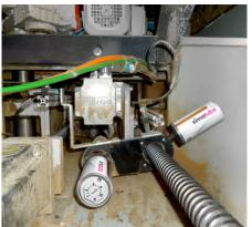
The spindle of a circular saw is reliably lubricated with two 125 ml simalube cartridges.
