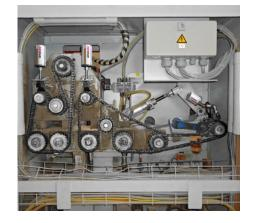
The chains of a cross-cut machine with roll feed are permanently lubricated using three simalube lubricators fitted with brushes and cleaned at the same time.
