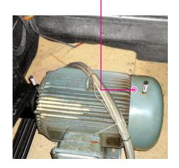
The electric motor of a chipping machine is lubricated in a sawmill.
