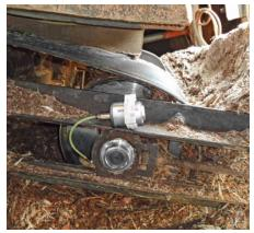
The Y-ball-bearing unit of a conveyor belt is continuously supplied with lubricant.
