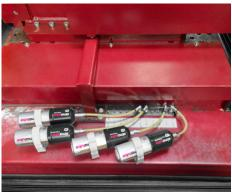
Four simalube IMPULSE connect pressure boosters lubricate the linear guides of a CNC machine by means of hose connections. Each IMPULSE can be controlled and configured individually with the simatec app.
