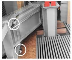
In a sawmill, the bearings of a chain conveyor are at an inaccessible height. These can be conveniently monitored thanks to the Bluetooth® connection to the simalube IMPULSE connect.
