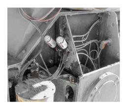
In a quarry, two simalube IMPULSE connect pressure boosters effortlessly overcome the counter-pressure of two bearings. These were also included in the simalube lubrication plan «Lubechart» via the simatec app.
