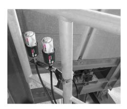
The lubrication points are at a dangerous height. They can be controlled conveniently from the ground with the simatec app.
