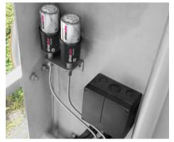
Due to permanently installed lubrication lines on a pool cleaner, two simulube IMPULSE connect are used. They overcome the back pressure and ensure continuous lubrication.
