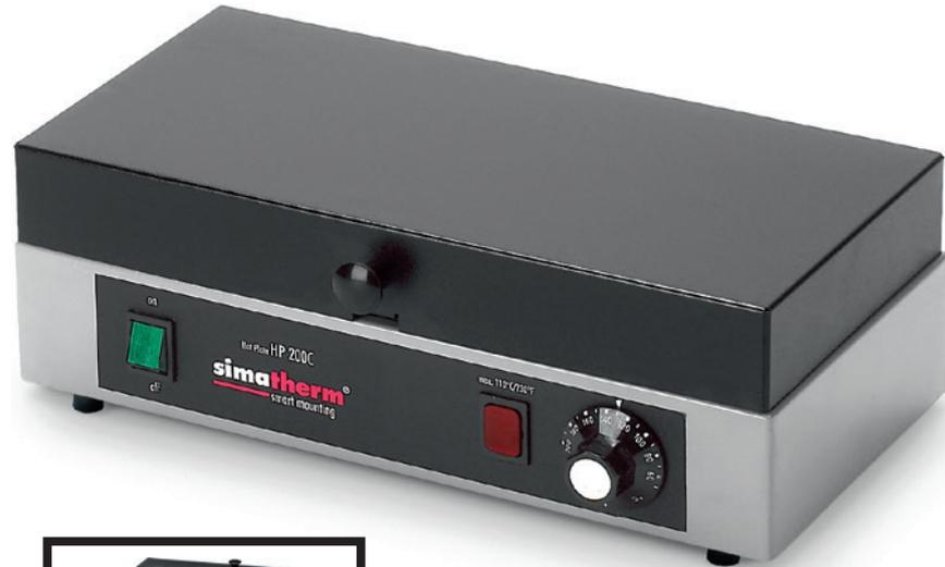
These electric hot plates with thermostat-controlled bearing heating are especially suited for heating small bearings or small machine parts. The temperature is infinitely adjustable from 50°C to 200°C.
