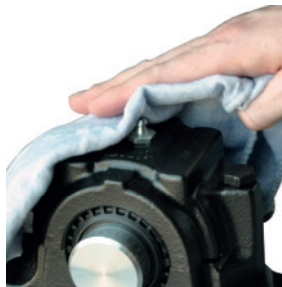
Clean lubrication point
