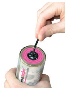
Activate calculated dispensing time with 3 mm Allen key
